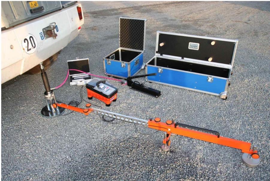
The AX01 Plate Load Test (or Plate Bearing Test) is an insitu site investigation field test used to determine the ultimate bearing capacity of the ground and the likely settlement under a given load. It is designed for measuring static loads on spread footings (e.g. to determine whether the ground has sufficient bearing capacity to support structures or temporary cranes or piling rigs), and for repetitive plate loading tests of soils and flexible pavement sub grades.
